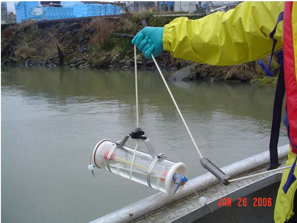
Photo #1: Looking at the Van Dorn sampler post-deployment with water column sample inside.
